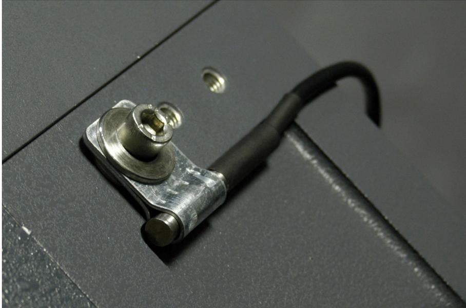
*Figure 2: Sensor Mount: Thermally Bonded*
